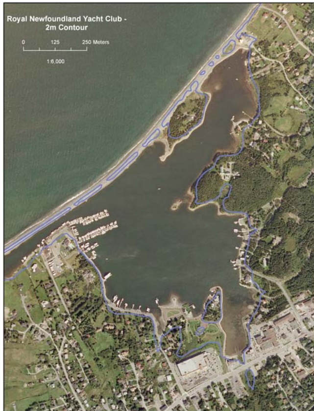
Plate 7. Vertical aerial photograph of part of the Town of Conception Bay South showing an extensive barachois beach system. This beach protects low-lying areas inland (2 m contour shown), much of which have been developed. Future relative sea-level rise, plus storm surge, could breach the barachois beach and inundate coastal properties.
