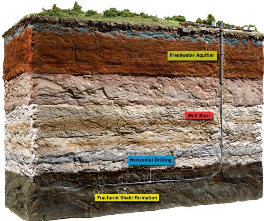
When we say the rocks are “tight”, we mean that they are impermeable. There are not enough cracks and pores in the solid rock to allow fluids or gases to move around. Hydraulic fracturing involves perforating the well casing at target depth 1 – 3 kilometers below the surface and then using water pumps to fracture the tight rocks and push sand into the new hairline fractures to hold them open.
